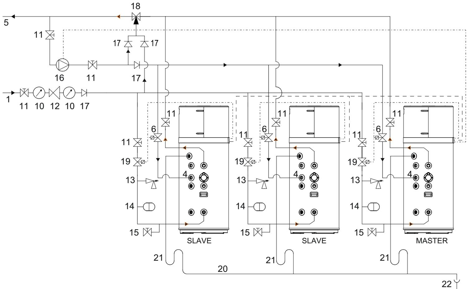
fig. 64 - Example of water system WITH thermostatic mixing valve (recirculation on unit water recirculation connection)
