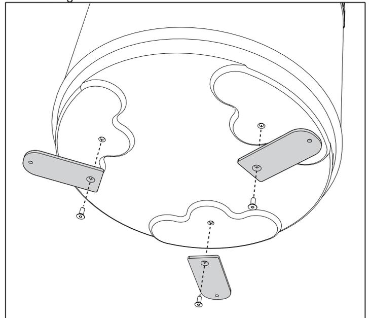
fig. 50- Fixing the brackets
