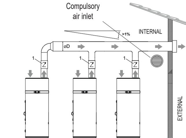
fig. 54 - Example of air discharge connection
